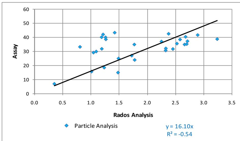
**Figure 6: Typical Results obtained from the analysis of individual particles showing that there exists a tenuous relationship between the surface and bulk analysis.**
