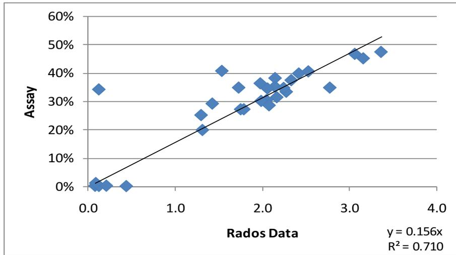
**Figure 5: Typical Results obtained from the analysis of individual particles showing a relationship between the surface and bulk analysis.**
