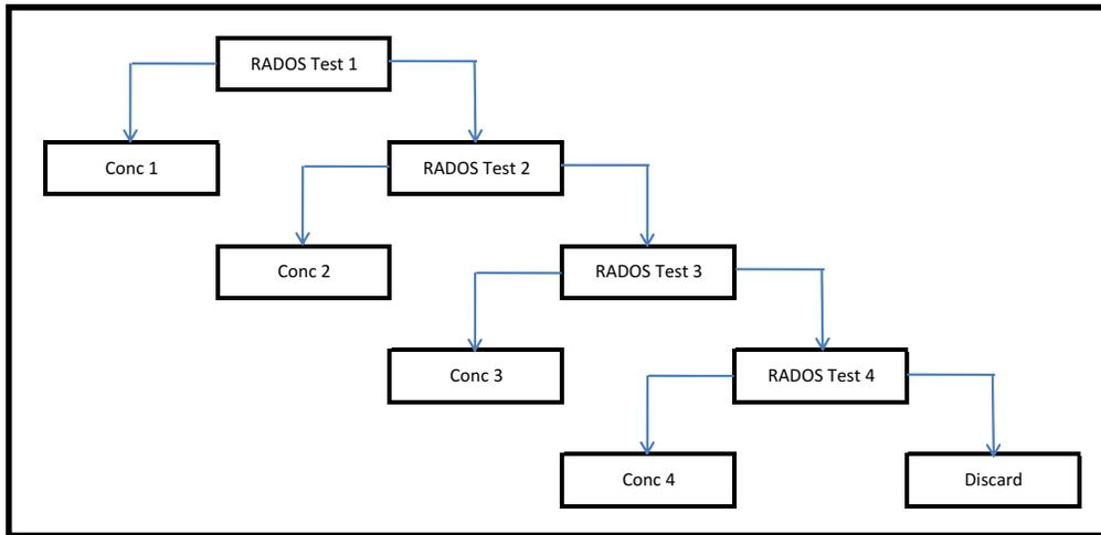
**Figure 8: Flow Diagram showing the Grade-Recovery Testwork procedure**
