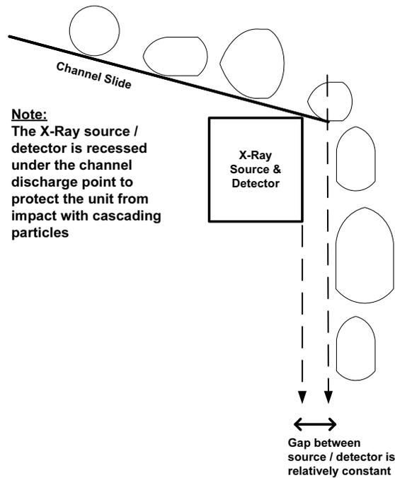
**Figure 3: Schematic view of the RADOS XRF Ore Sorter.**
