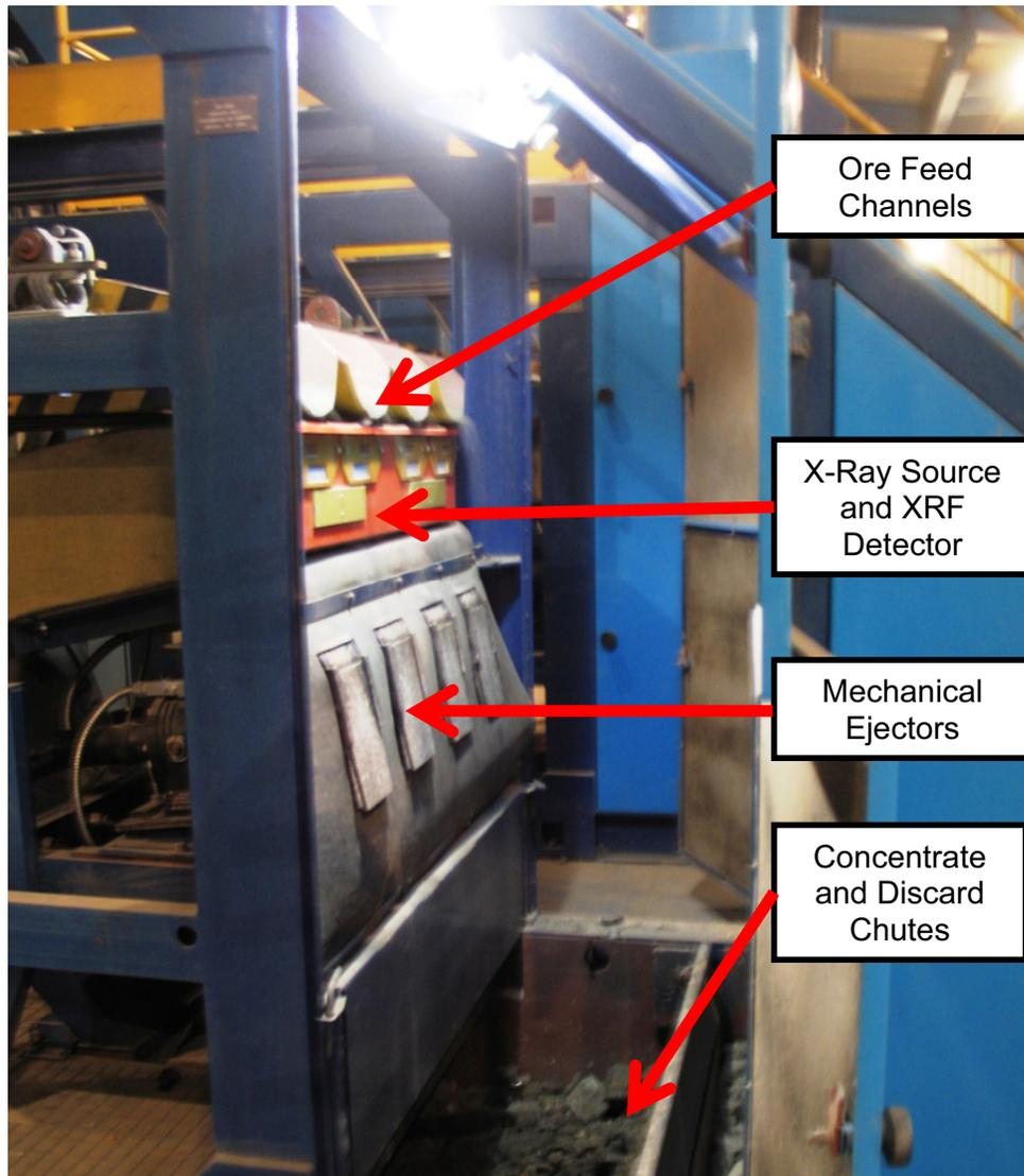
**Figure 2: Layout of the RADOS XRF Ore Sorter**
