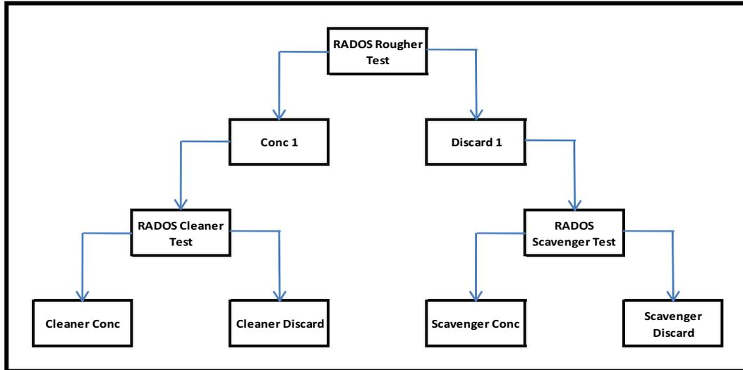
**Figure 10: Block Flow Diagram showing the test procedure used to measure the efficiency of the RADOS Sorter**
