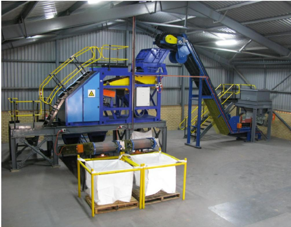
**Figure 4: The Rados XRF Ore Sorter at Mintek**
