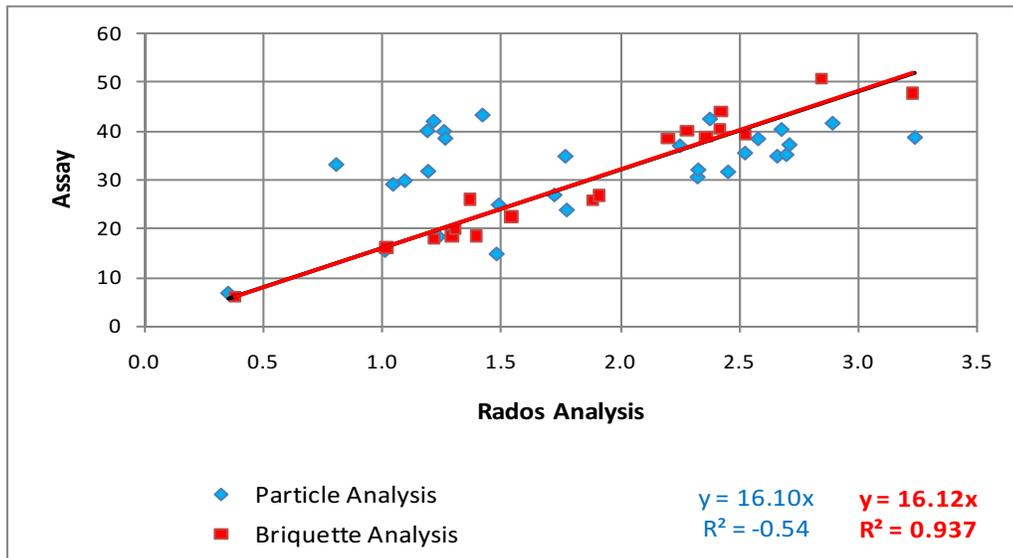
**Figure 7: A comparison of the results obtained from the analysis of individual particles and briquettes manufactured from the pulverised residues from analysis.**
